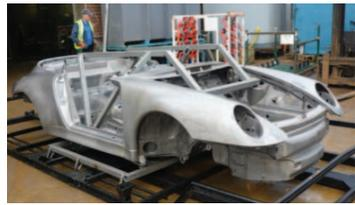
advanced corrosion protection in the form of electrophoretic coating (or e-coating) to prevent its return.
