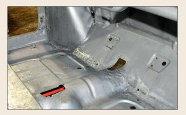
**18** Repairs complete, return the shell and parts to SPL to repeat the final stages of the cleaning process to remove any additional grease and unwanted contaminants. After having the shell acid dipped and cleaned, Derek's Mini Centre has done a fantastic job on the restoration of this Mk2 shell and it has now returned for the final clean.
