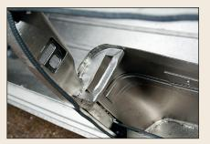
specialist and have the nickel plating applied. Although not cheap at  $\pounds 2,500$  including the acid dip, SPL reckon the procedure will offer the best possible protection against further corrosion as it penetrates every part of the shell, as can be seen on this cross-sectioned Clubman Estate. It will come with a three-year anti-perforation warranty.
