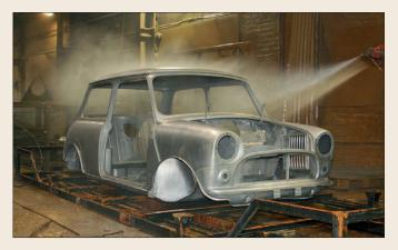
**16** The shell or parts are dipped for a final time in a neutralisation diprocess to remove any leftover acidic traces from the previous dip. The highly-alkaline solution of the final dip reaches inside all nooks and crannies to ensure a thorough neutralisation of the steel, even in the bits you can't see or reach. The pressure jet is used again to clean up the components. A chemical reaction between the steel and the solution leaves a shiny metallic finish.
