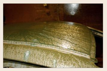
$\mathbf{10}^{\text{The shell}}$  and parts need to be pressure washed once again to remove the green residue which remains after the first submersion.
