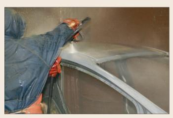
**11** The pressure jet contains a preservative. Water alone is avoided in the plant so that any surrounding bare metal parts do not rust. Particular attention is paid to the seams and crevices, especially on a Mini.
