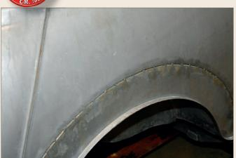
12Removing all of the organic contaminants may reveal past repair work that you didn't even realise existed, such as this rear arch repair which would have been hidden with a skim of filler under the paint. Thankfully, this is a good quality repair on this shell. On others you may find all manner of bodges.
