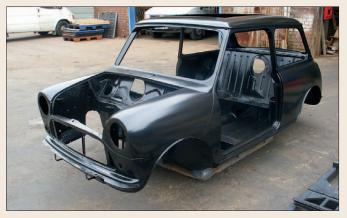
**19**<sup>EN</sup> plating or electrophoretic-coating (e-coating) is the next best e-coated after having the full acid dip treatment. Because of the full-emersion technique of the EN-plating and e-coating procedure, shells will be treated inside the box sections too. E-coat is the finish you'll recognise from most aftermarket Mini panels.
