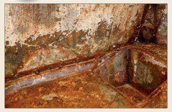
$02^{\rm Every}$  panel is red rusty from being stripped and left to the elements of the plaqued with holes. You'd be forgiven for thinking this is scrap, but with the value of solid Mini bodyshells increasing, a shell like this is still worthy of repair.
