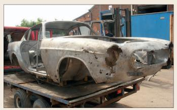
**15** The same cannot be said of rusty bits. The owner of this Volvo **15** P1800 may be surprised by the end result. At least the true extent of the damage is now visible. Otherwise, the rust may have been ineffectively patched-up or gone unnoticed and continued to corrode its way through the shell with potentially dangerous or expensive consequences.
