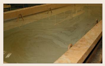
**07**The first chemical bath contains a secret alkaline hydrocarbon solution, heated to 85-degrees C, to break down any remaining 'heavy organic contaminants'. When the shell is fully submerged in this special chemical solution for a few hours, any filler, sealants, waxes and grime are broken down and removed. Paint will also be stripped back, leaving a completely bare-metal shell from the inside out.
