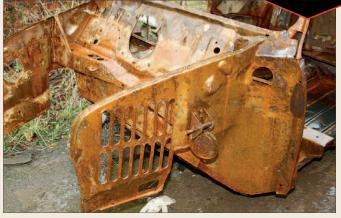
**O3**The wings and many of the front panels have already been removed. If you can see that panels will definitely need to be replaced you may as well remove them prior to dipping, as long as it doesn't affect the structural integrity of the shell. All of the glass, interior, running gear and electrics will need to be removed.
