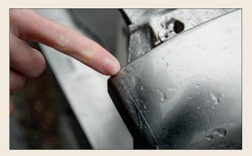
**14** If you are concerned about your Mini's steel being eroded away by the chemicals used in this process, check out this Clubman front wing. The chemicals are so gentle on the metalwork that these scuffs caused by pre-paint preparation at the factory are still present on the panel.
