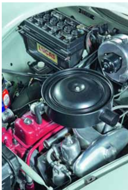
The B-series engine was rebuilt and married to a Type-9 gearbox. The interior needed a jolly good clean.
