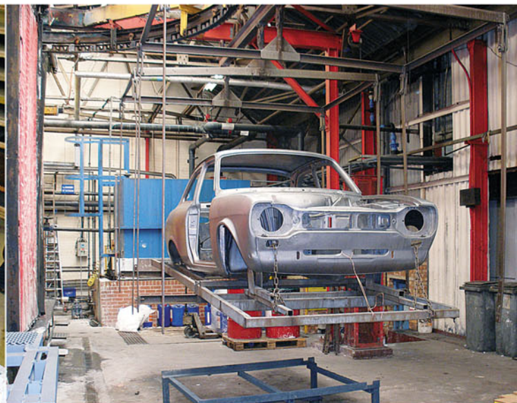
When going to be e-coated the shell is mounted on a cradle, chained down, wired and earthed ready for the 19 stages that are ahead
