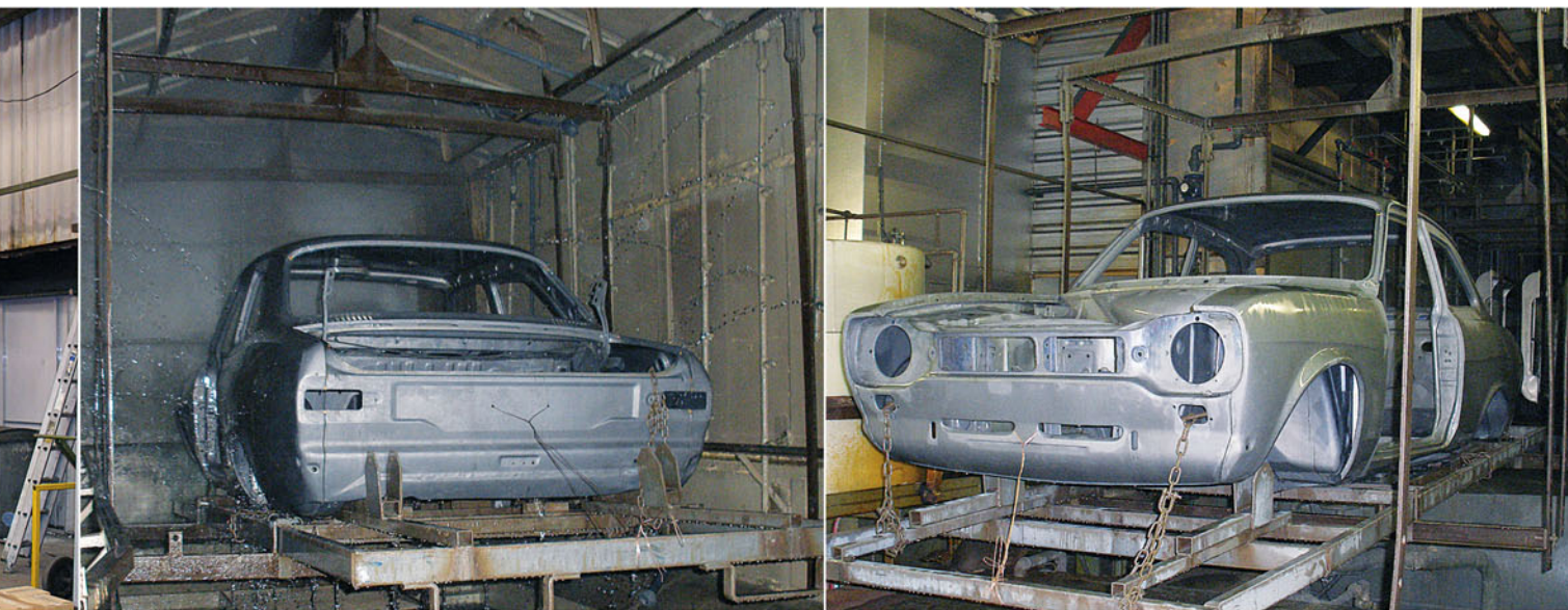
The shell gets washed many times in a variety of solutions to prepare it for the electrostatic dipping process. It's never been so clean!
