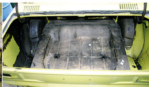
Panels before and after dipping – like new! Bulkhead looked a bit scabby, the acid reveals some minor holes. Ziebart in boot no problem!
