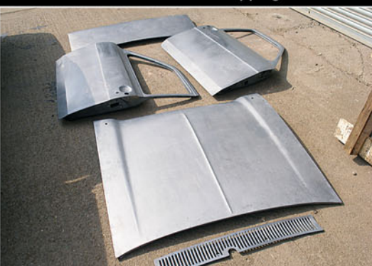
Panels before and after dipping – like new! Bulkhead looked a bit scabby, the acid reveals some minor holes. Ziebart in boot no problem!
