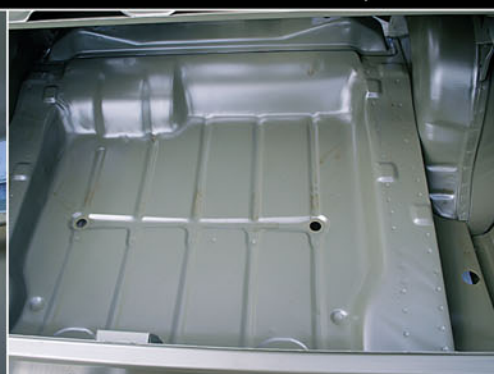
Panels before and after dipping – like new! Bulkhead looked a bit scabby, the acid reveals some minor holes. Ziebart in boot no problem!
