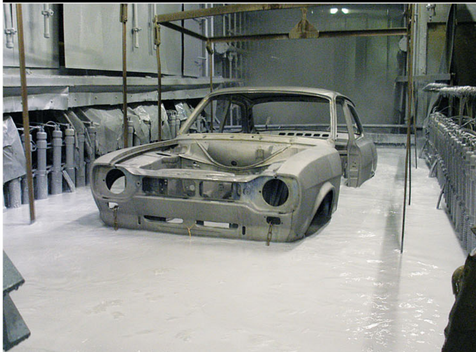
Below: It's almost like something out of the Terminator movies... The shell is lowered into the e-coat solution and stays there for 5 minutes
