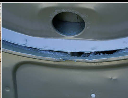
Panels before and after dipping – like new! Bulkhead looked a bit scabby, the acid reveals some minor holes. Ziebart in boot no problem!
