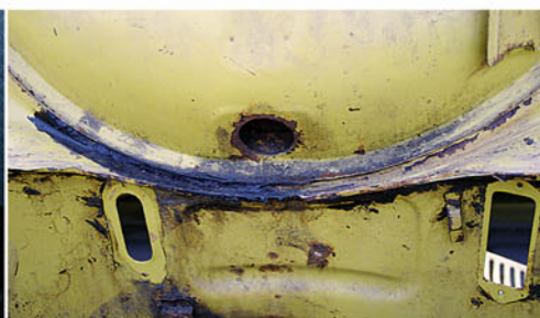
Panels before and after dipping – like new! Bulkhead looked a bit scabby, the acid reveals some minor holes. Ziebart in boot no problem!
