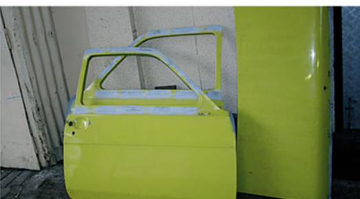
Panels before and after dipping – like new! Bulkhead looked a bit scabby, the acid reveals some minor holes. Ziebart in boot no problem!
