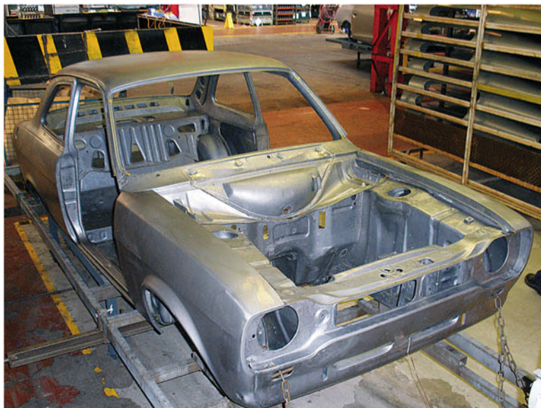
When going to be e-coated the shell is mounted on a cradle, chained down, wired and earthed ready for the 19 stages that are ahead
